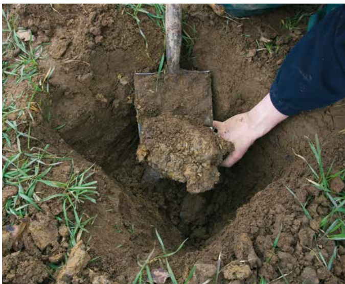
Figure 7. Clay subsoil showing vertical fissuring
