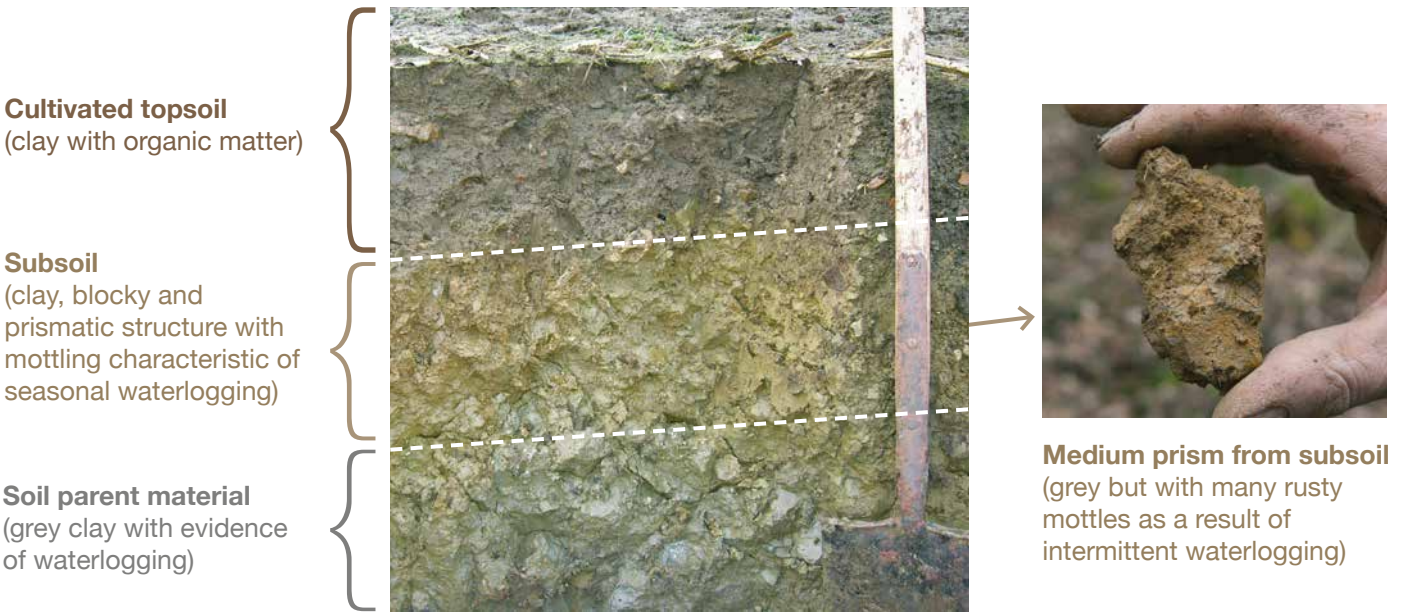
Figure 2. Soil profile showing characteristic horizons. This is a surface-water gley soil showing gleying as a result of waterlogging. The clay soil is relatively impermeable and, therefore, anaerobic conditions occur during excess rainfall
